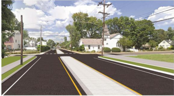
S.R. 0413 (Pine Street) Traffic Calming - Option 2 (Median with Left Turns Allowed)
